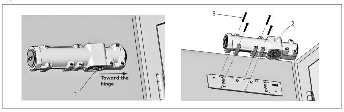
NOTE: Orient pinion (1) closest to hinge.
